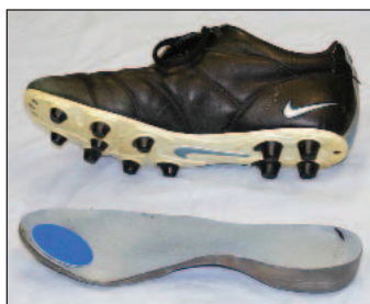
Figure 1. Low-friction interface patch applied to the toe area of a soccer shoe insole.
