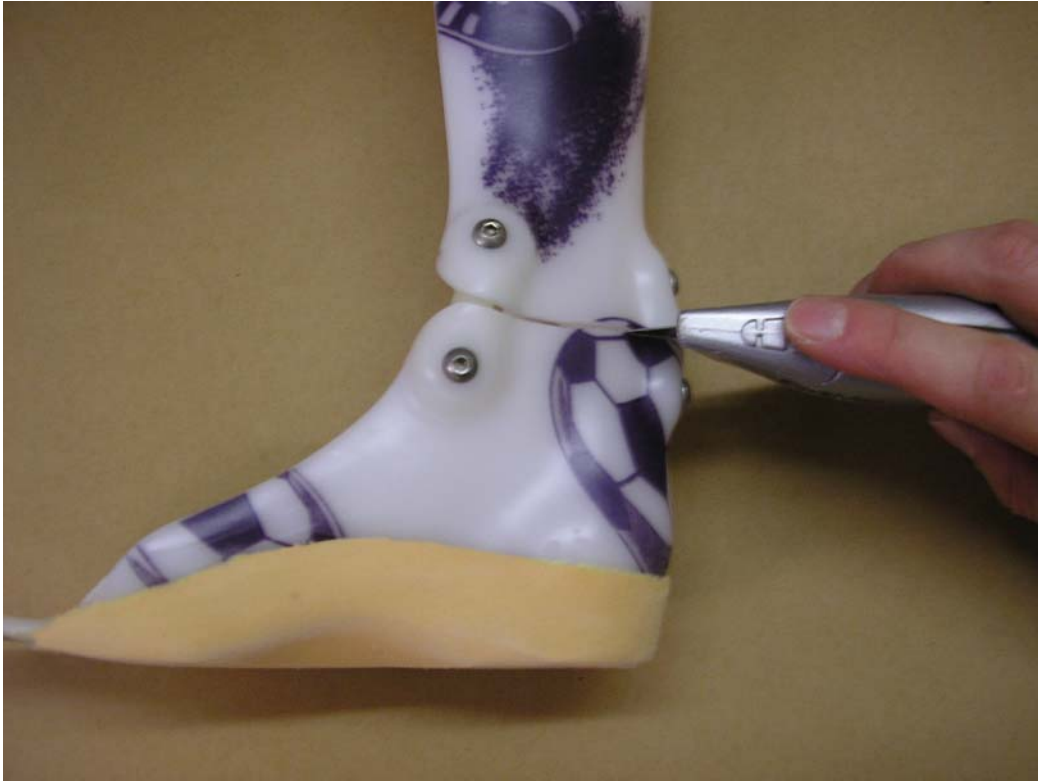
Figure 3(a) Cutting through the posterior flexure joint.
