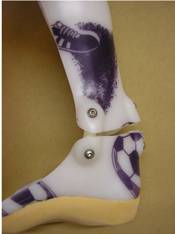
Figure 3(b) The articulation and plantarflexion stop.
